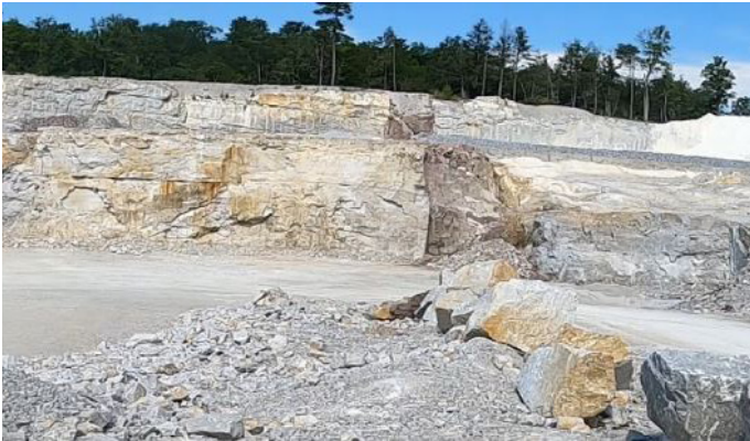
The rock face, with the dark brown contaminated stone on the right of the lighter high-quality production stone
